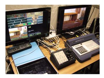
In most of our bldgs our control booth is setup in the satellite equipment room with CAT5 cables permanently installed through the attic to each camera, but this particular bldg required us to setup in the overflow area.
