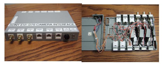
One CAT5 cable is used to connect all signals to and from each camera. A custom box was constructed to get all the signals to/from CAT5 .
